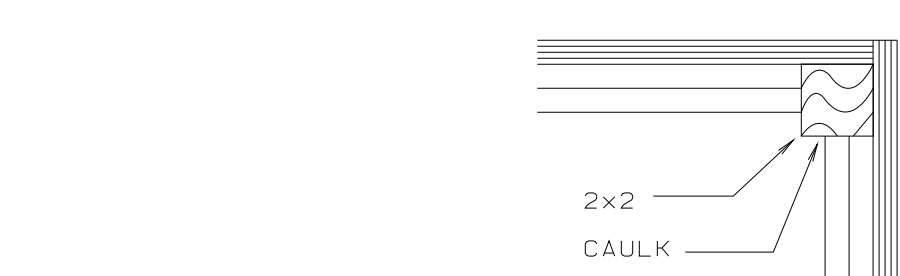
3 INTERIOR CORNER SIDING DETAIL.
